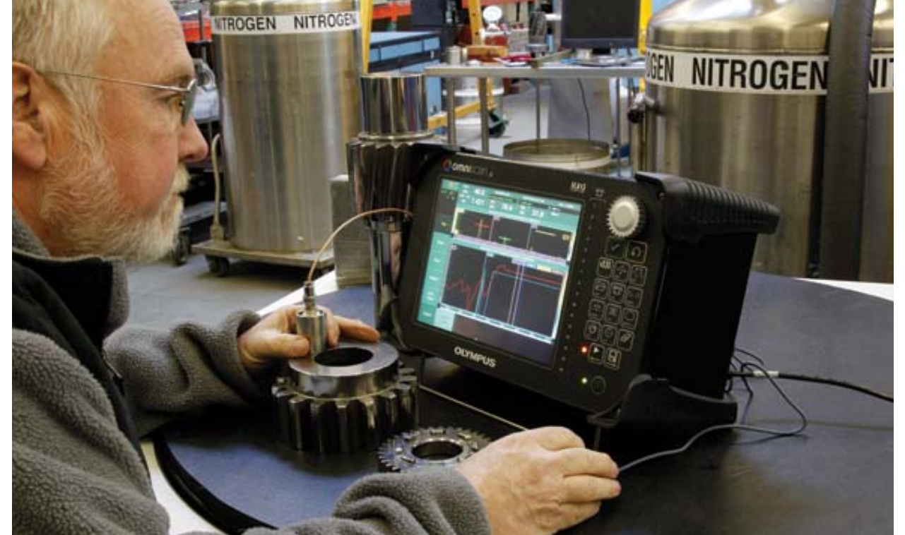
Victor can measure the quality of engine parts using innovative electromagnetic acoustic techniques; then evaluate how they're improved employing cryogenics.
